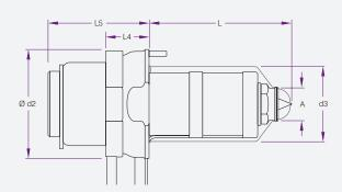
With two heaters the SX nozzle is perfectly suited for all single nozzle applications. Independently controlled heater zones provide uniform temperature distribution along the length of the nozzle, making it ideal to process difficult plastics.
