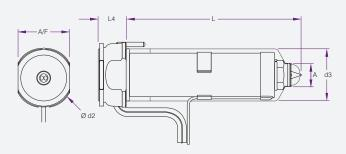
Low moulding temperature and pressure, excellent temperature consistency and front loading capabilities, that's the Mastip MX nozzle, specifically designed for multi cavity manifold systems and hot halves. The MX nozzle is suited for small to medium applications in all types of markets. It is able to process a wide range of plastics, from the easy ethylenes to tough engineering resins.
