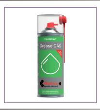
H-1 approved for use in food processing equipment where incidental contact with food may occur. They are designed to provide superior performance at low and elevated temperatures (-40°C~200°C) and during periods of infrequent lubrication in food processing applications. Foodmax Grease CAS can be used for general lubrication, slide ways, chains and high load bearings in the food industry.
