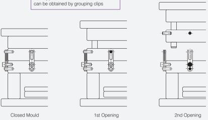
Mat.: 1.8159 Hardened: 45 ± 3HRC Patented System No pocket machining required as needed with other similar products on the market. Minimum space required for installation. Reduces costs compared to conventional mechanisms. Offers a standard solution to the molder.
