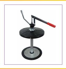
The 20kg grease pump is suitable for bulk filling of manual or electric hand grease guns. With a durable cast aluminium alloy pump outlet body, it allows for the fast reload of grease guns, taking less than a minute. The nipple allows bulk fill to valve with diameters of 9mm and 12.5mm. Comes standard with a Rubber follower plate.
