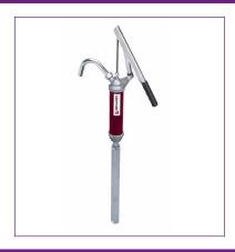
The Lever Action Barrel Pump is a telescopic suction tube for eitehr 60L or 205L drums. Comes with 1 - 1/2" & 2" bung adaptors. Can pump up to 500ml per stroke, depending on viscosity. Wetted materials: steel, aluminium, zinc, brass, NBR, viton and suitable for lubricating oils and service fluids.
