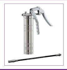
One hand grease gun with zinc plated steel barrel to suit 400g shuttle type cartridges, and an ergonomically designed pistol grip. Fast and clean loading and unloading without opening the gun, eliminating any contamination.
