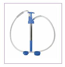
Designed for dispensing most service fluids including engine, gear, transmission, hydraulic and some engine coolants from 20L - 25L drums. An extendable suction tube and two additional bung adaptors ensure that the expanding range of different size and types of drums are easily catered for. An extra-long clear delivery hose gives easy identification of the fluid type and allows better reach into difficult areas.
