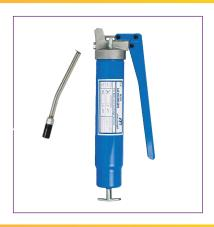
A lever-action grease gun designed for high pressure / high volume greasing and can easily clear blocked or damaged grease nipples. The grease gun features a durable die cast aluminium head, a heavy gauge steel barrel and a heavy duty follower assembly to handle a wide range of grease viscosities. Suits 450g grease cartridges, bulk filling or MacNaught J3 transfer loading.
