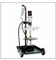
The complete set of fluid transfer accessories gives the end user a trouble-free using experience. The standard model is composed of 50:1 pump, trolley, follower plate and drum over, 4 meter of 1/4" connection hose, 'Z' swivel and control gun with a working pressure of up to 8700psi.
