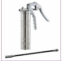
One hand grease gun with zinc plated steel barrel to suit 400g shuttle type cartridges, and an ergonomically designed pistol grip. Fast and clean loading and unloading without opening the gun, eliminating any contamination.
