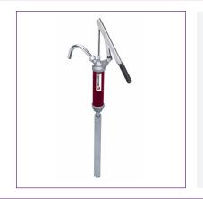
The Lever Action Barrel Pump is a telescopic suction tube for either 60L or 205L drums. Comes with 1 - 1/2" & 2" bung adaptors. Can pump up to 500ml per stroke, depending on viscosity. Wetted materials: steel, aluminium, zinc, brass, NBR, viton and suitable for lubricating oils and service fluids.
