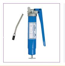
A lever-action grease gun designed for high pressure / high volume greasing and can easily clear blocked or damaged grease nipples. The grease gun features a durable die cast aluminium head, a heavy gauge steel barrel and a heavy duty follower assembly to handle a wide range of grease viscosities. Suits 450g grease cartridges, bulk filling or MacNaught J3 transfer loading.
