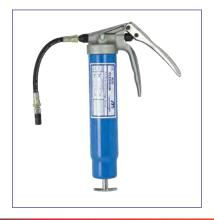
A classic grease gun that incorporates a unique variable stroke piston and valve arrangement for true one handed operation and can produce increased pressure through short strokes or high volume shot using a full stroke. Pistol-grip design to suit 450g grease cartridges, bulk filling or J3 grease transfer pump loading.
