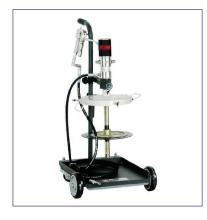
The complete set of fluid transfer accessories gives the end user a trouble-free using experience. The standard model is composed of 50:1 pump, trolley, follower plate and drum over, 4 meter of 1/4" connection hose, 'Z' swivel and control gun with a working pressure of up to 8700psi.
