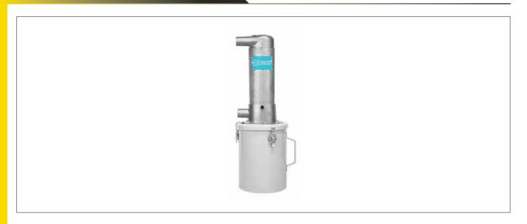
Designed to eliminate powder and fines contamination from plastic pellets, the ARV 38 De-Duster can be installed into any material line, to ensure more stable plasticising and eliminate product defects caused by incomplete melting.
