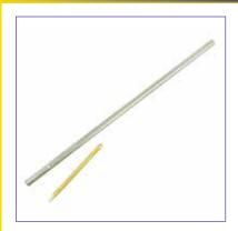
A simple but effective tool for removing over packed plastic material from sprues or hot runner systems. The knock-out bar combines a tough steel rod with threaded brass replaceable tips that prevent damage to the mould surface.
