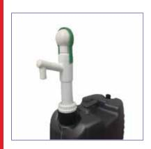
Ezy-Action food grade hand -operated piston pump is made of polypropylene for resistance to chemicals, dispenses liquids at a rate of 15oz. per stroke, and is suitable for dispensing viscous fluids, hard acids, or alkali cleaning chemicals
