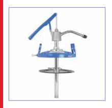
Designed for fast, easy bulk filling of grease guns. This provides an economical solution for refilling most standard grease guns from bulk pails instead of purchasing more expensive grease cartridges. The sealed system also keeps grease free from contamination. A height adjustable lid and pump assembly offers compatibility with several different size grease pails up to 20kg.
