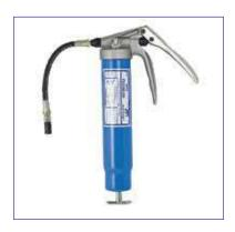
A classic grease gun that incorporates a unique variable stroke piston and valve arrangement for true one handed operation and can produce increased pressure through short strokes or high volume shot using a full stroke. Pistol-grip design to suit 450g grease cartridges, bulk filling or J3 grease transfer pump loading.
