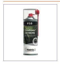
This product is based on highly polar biodegradable ester base oil and is inhibited against oxidation to give a long wet film life at high temperatures up to 285°C. Foodmax Extreme is designed for the lubrication any moving part in the food, cosmetic, pharmaceutic, textile, glass, steel, and wood industry. Foodmax Extreme possesses outstanding anti wear capacity and will reduce wear on
