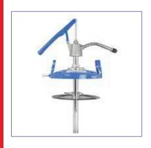
Designed for fast, easy bulk filling of grease guns. This provides an economical solution for refilling most standard grease guns from bulk pails instead of purchasing more expensive grease cartridges. The sealed system also keeps grease free from contamination. A height adjustable lid and pump assembly offers compatibility with several different size grease pails up to 20kg.
